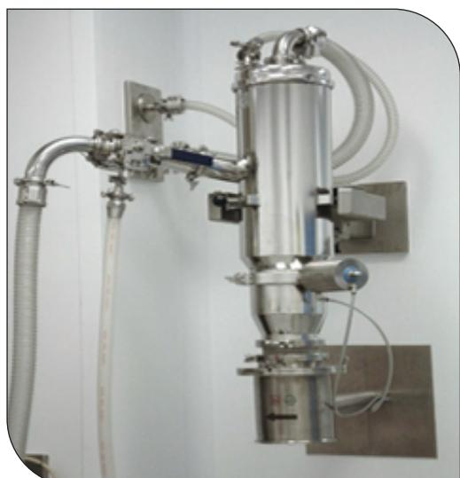
Post FBP, to transfer granules / pellets to next phase of blending, compression, capsule filling or sachet packing; dust free solutions customised to user need are available from Genesis.
