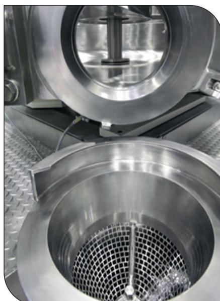
Under Driven Cone mill with round blade and option of square, round sieves
