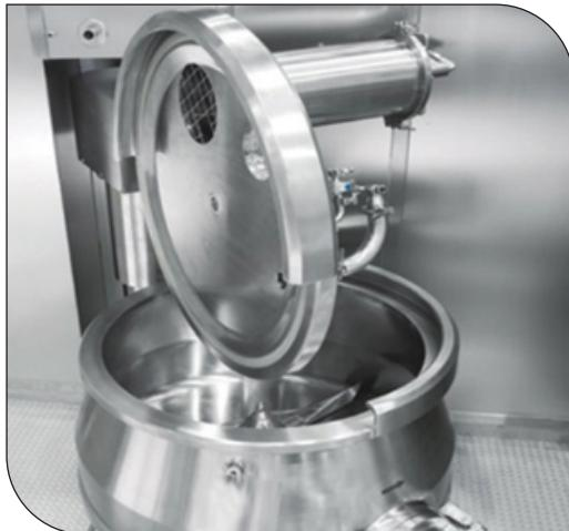
The processing of highly flammable solids or organic solvents requires special measures for explosion protection. Your safety is guaranteed by reliable protection procedures such as explosion shock-resistant design, a technique mainly used for mixer-fluid bed combinations.
