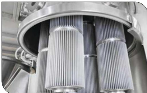
Special WIP SS cartridge filter bag provided for containment application with Air blow cleaning system & auto lowering with pneumatic telescopic cylinder
