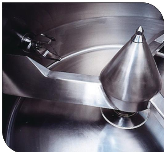
Unique Tangential elevated tip impeller for unique mixing pattern
